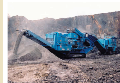
▲ An 1180 Premiertrak feeding 1300 Maxtrak producing type 1 sub-base at 300tph / 330 Stph
