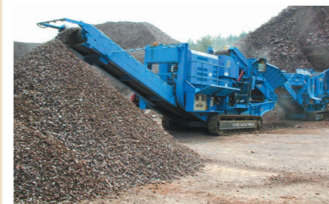
▲ 1165 Premiertrak working with a 1000 Maxtrak to produce 40mm / 1 1/2" sub-base on a basalt application.
