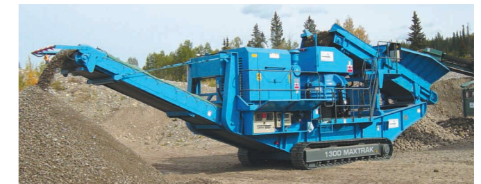
▲ HIGH CAPACITIES The 1300 Maxtrak is capable of capacities up to 350 tph / 386 stph depending on the application.
