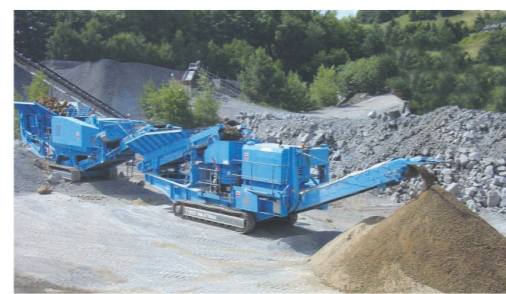
▲ The 1000 Maxtrak has been designed to maximise throughput, reduction and product shape in a wide range of quarrying applications.
