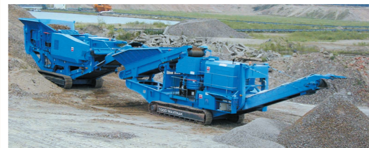
▲ Two stage crushing showing a 1165 Premiertrak feeding a Maxtrak 1000 producing sub-base material.
