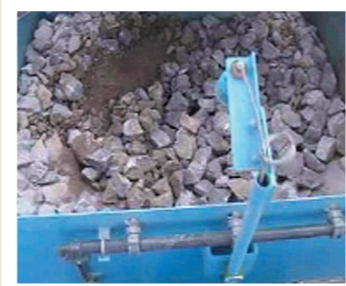
▲ FEED BOX Fabricated to control choke feed with level probe to monitor the flow of material through the crusher.
