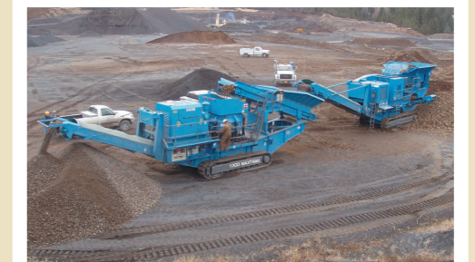
▲ An 1180 Premiertrak feeding a 1300 Maxtrak to produce road base material.
