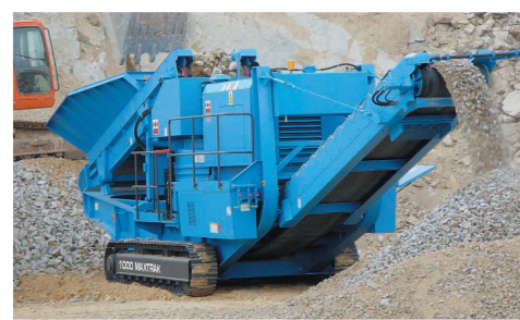
▲ HIGH PRODUCTION CAPACITY A Terex® Pegson 1000 Maxtrak on a limestone application.
