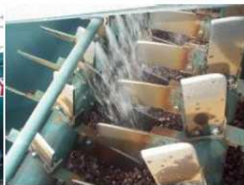
Axles with high tensile and quickly replaceable blades
